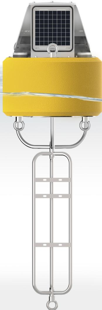
The NexSens **CB-150** Data Buoy is designed for deployment in lakes, rivers, coastal waters, harbors, estuaries and other freshwater or marine environments. The floating platform supports both topside and subsurface environmental monitoring sensors including weather stations, wave sensors, thermistor strings, multi-parameter sondes, Doppler current profilers and other monitoring instruments.
