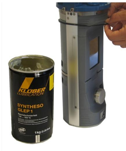
Figure 8-5 Lubricate O-rings with grease. (Klüber Lubrication Syntheso Glep 1 or similar synthetic grease).
