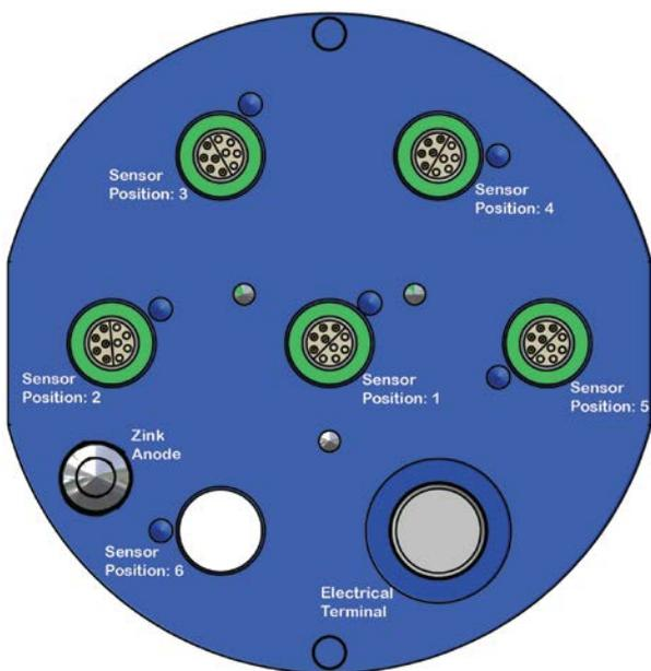
**Figure7-8 Top view of Top-end plate; Sensor Positions.**
