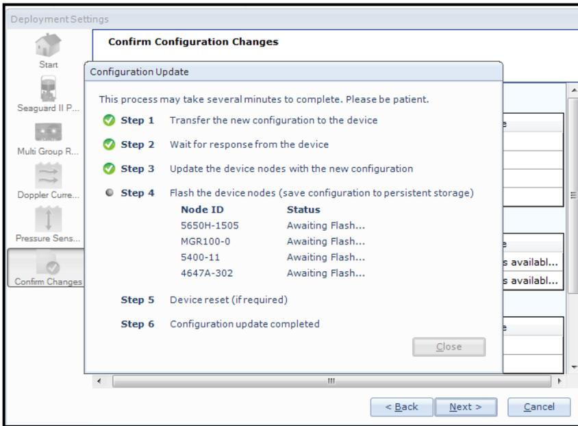
Figure 3-16: Deployment settings configuration update
