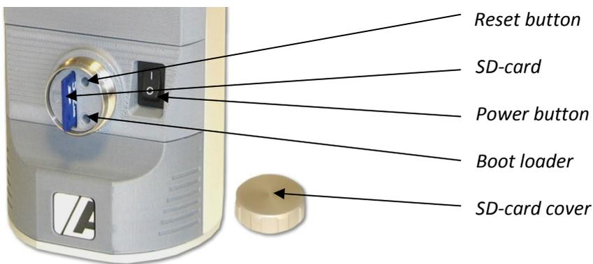
Figure 1- 3 SD-card slot
