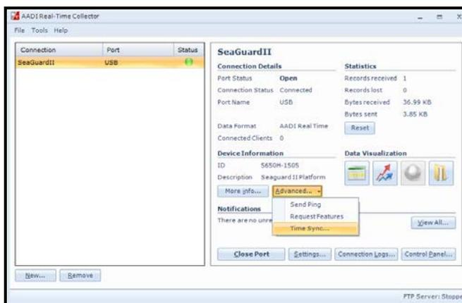
**Figure 3-29; access Time Sync functionality**
