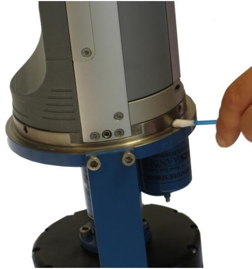
Figure 8-2 Clean O-ring seating; instrument up-side-down.
