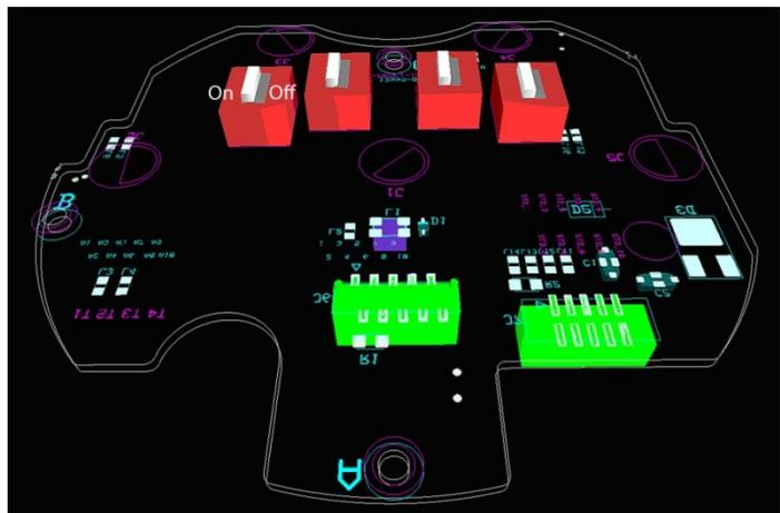
**Figure7-9 Drawing of HUB with 4 red Dip Switches at the back. AiCaP sensors installed: Switch to the right (off-position), Analog sensors: Switch to the left (on-position).**
