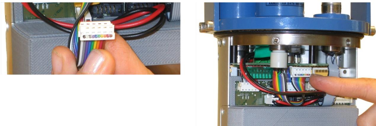
**Figure7-14** Connect the patch cable to HUB plug J6.
