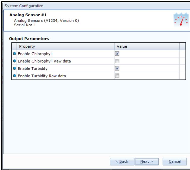
Figure 3-18 Analog Sensor
