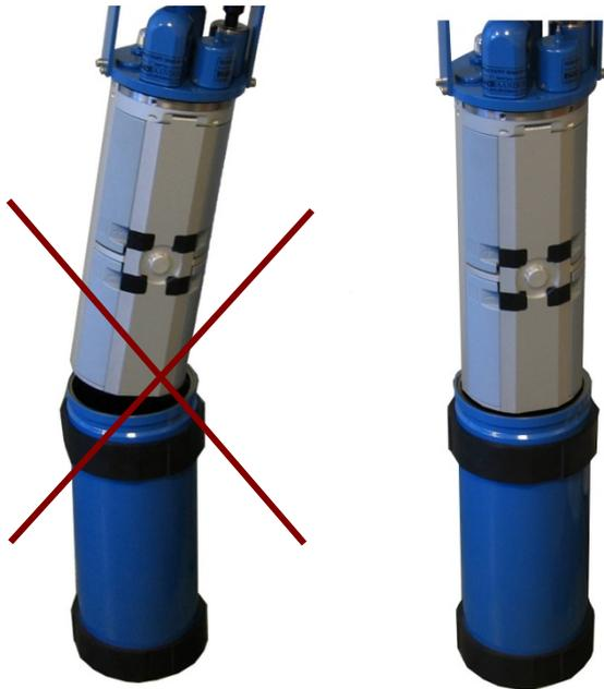
**Figure7-1 Insert Instrument into Pressure Case.**
