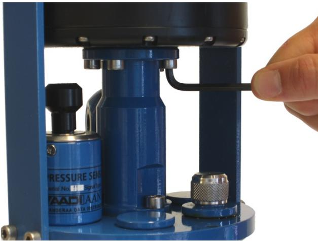
Figure7-15 Connect the ZPulse DCS / DCPS.
