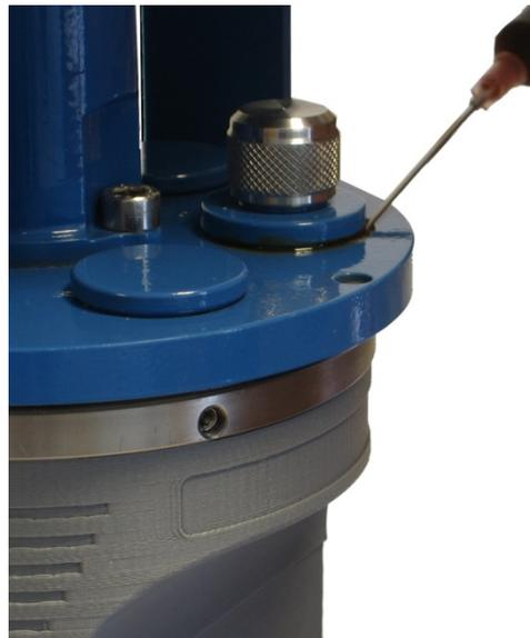
Figure 8-4 Add Tectyl® around sensors and sealing plugs.
