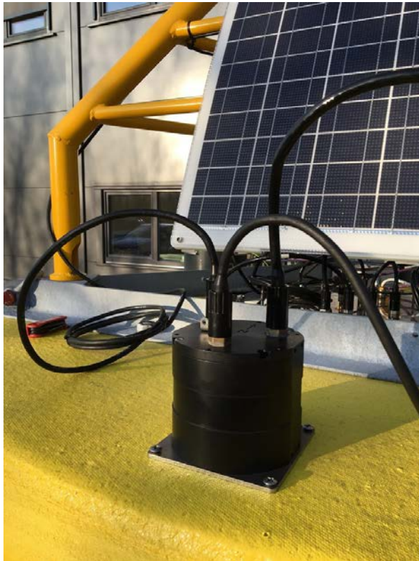
Figure 9-4: Sensor mounted with horizontal mounting plate
