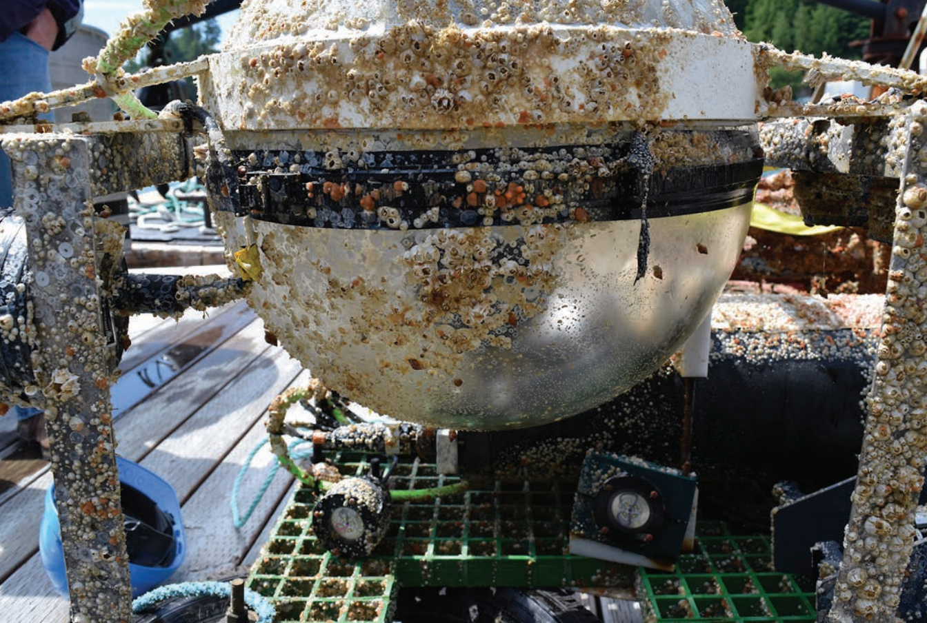
Figure 6: Camera sphere exhibiting signs of reduced fouling due to incidental UV exposure. UV test instruments located bottom right corner of image. Image used with permission from Ocean Networks Canada Innovation Centre.
