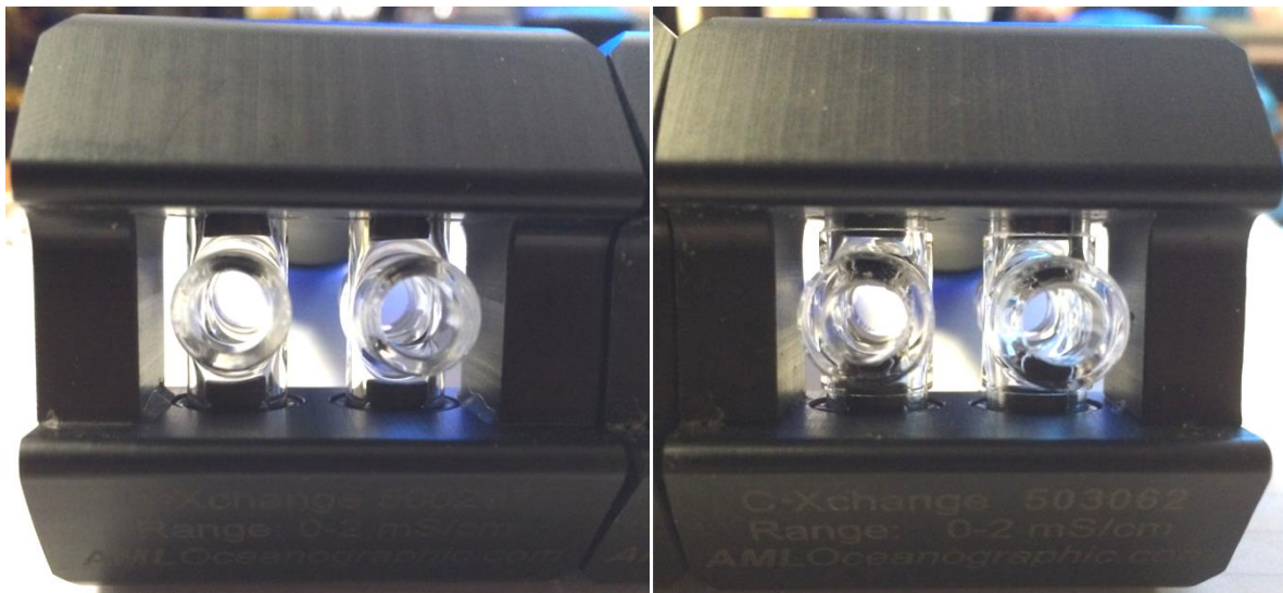
Left: Borosilicate glass cross tubes. Right: Fused quartz glass cross tubes. Note the thicker glass tubes on the right (fused quartz) sensor.
