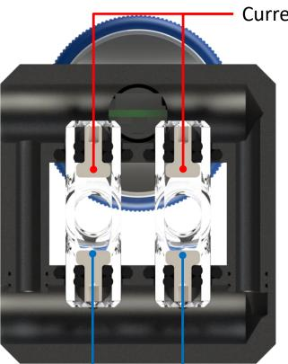
Current Electrodes (create the electrical field)
